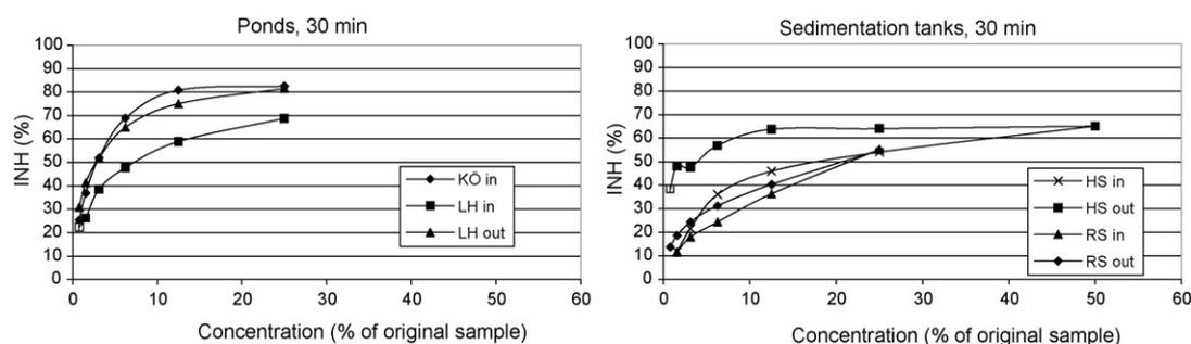
Fig. 6. Concentration response curves for the sediment in the ponds and sedimentation tanks after 30 min incubation.
