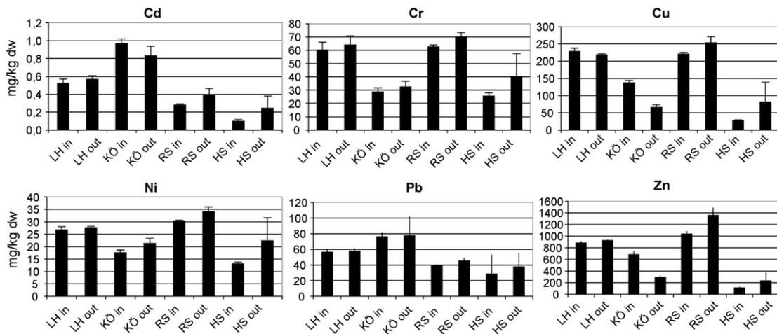
Fig. 3. Heavy metal sediment concentrations (with standard deviations) in the ponds and the sedimentation tanks (mg/kg dw).
