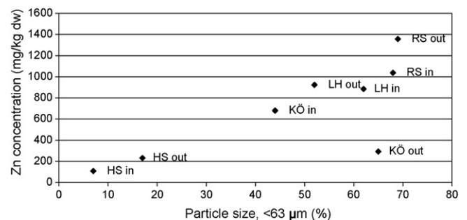
Fig. 4. Relationship between total Zn concentration and percentage of particles less than 63  $\mu\text{m}$  for all sediment samples.
