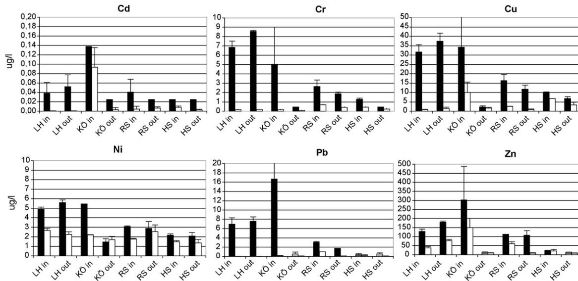
**Fig. 1.** Total and dissolved water heavy metal concentrations (with standard deviations) in ponds and sedimentation tanks ( $\mu\text{g}/\text{l}$ ).
