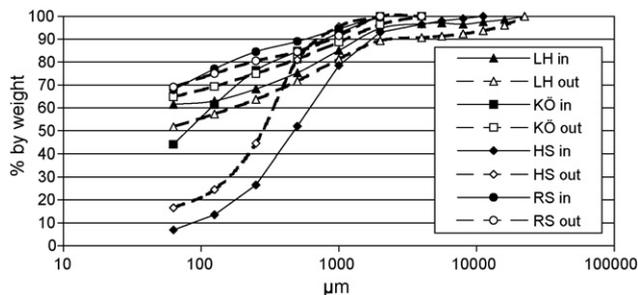
**Fig. 2.** Particle-size distribution curves for the inlet and outlet sediment samples from ponds and sedimentation tanks.
