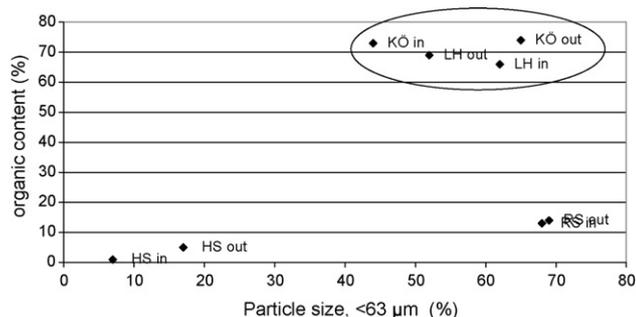
**Fig. 5.** Correlations between sediment organic content and the percentage of particles finer than 63 µm.
